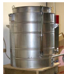
New Syrup Re-Heating & Filling Unit
